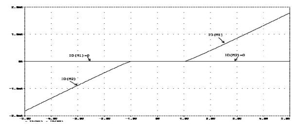
The transient analysis shows that the dead zone causes a distortion in the output waveform.
