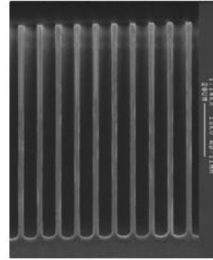
cross section of a silicon wafer demonstrating trenches that can be fabricated using DRIE tech
